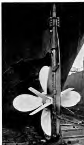
View of the contrapropeller installed on the steamship Norfolk of the Coastwise Transportation Corporation by Todd Shipyards Corporation.
